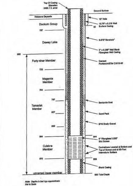
Figure L-12 As-Built Configuration of Well WQSP-6As-Built Configuration of Well WQSP-3
