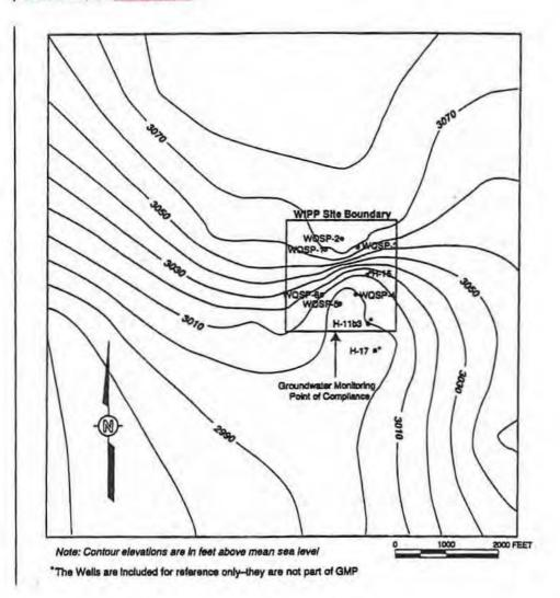
Figure L-9 As-Built Configuration of Well WOSP-3WIPP OMP Monitor Well Locations and Potentiometric Surface of the Culobra Near the WIPP
