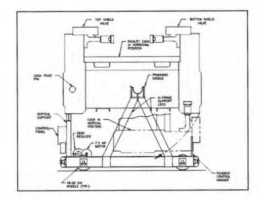
Figure A2-14 Facility Cask Transfer Car (Side View)
