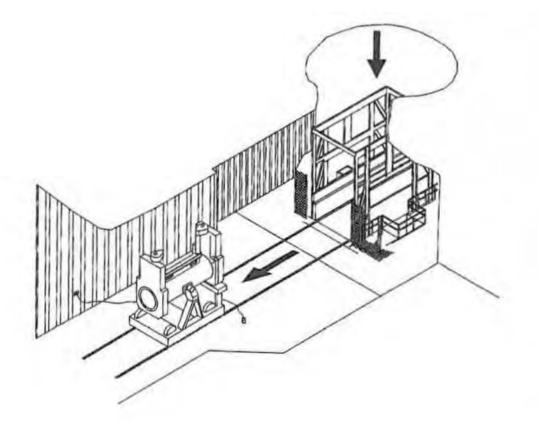
Figure A2-16 RH TRU Waste Facility Cask Unloading from Waste Shaft Conveyance
