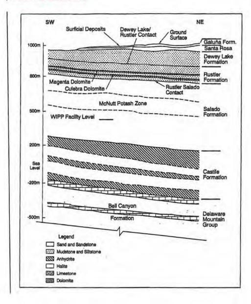
Figure L-4 Generalized Stratigraphic Cross Section above Bell Canyon Formation at WIPP Site Generalized Stratigraphic Cross Section above Boll Conven Formation at WIPP Site
