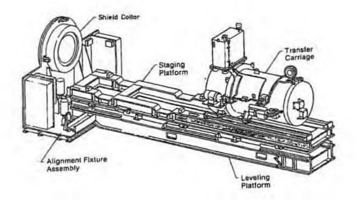
Figure A2-15 Horizontal Typical Emplacement and Retrieval Equipment
