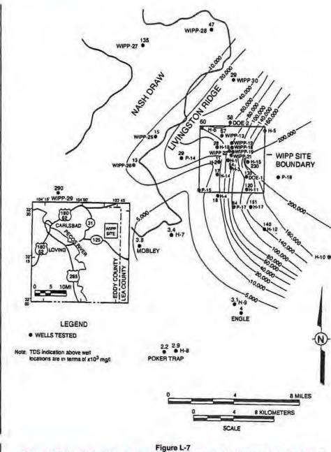
As-Built Configuration of Wall WOSP-17atal Dissolved Solids Distribution in the Culation
