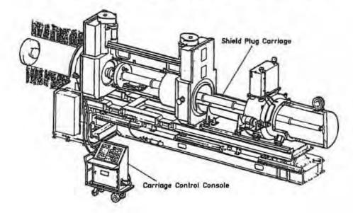
Figure A2-18 Installing Shield Plug
